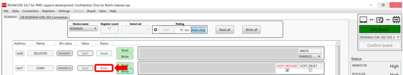
**Figure 23: "Error" status when no I<sup>2</sup>C communication is present**
