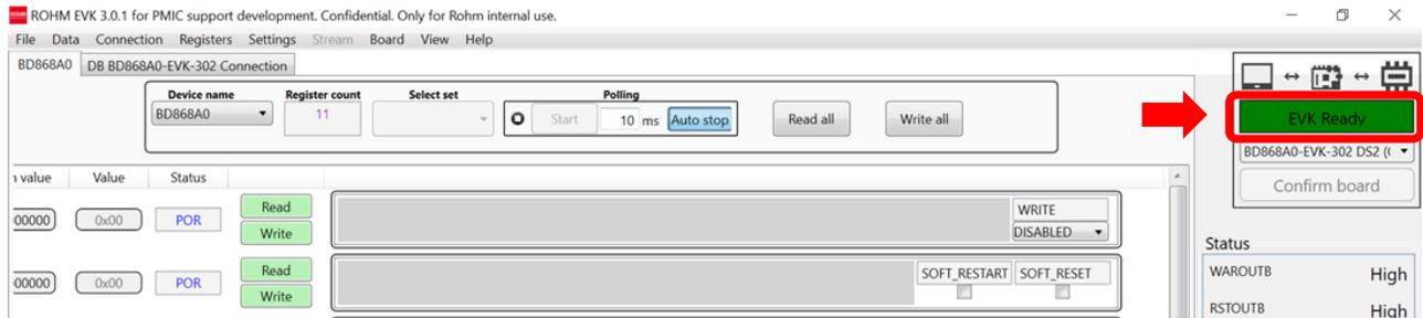
**Figure 12: Communication information in main page of GUI tool**
