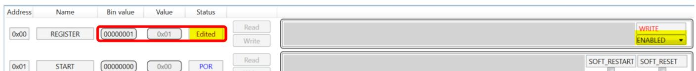
**Figure 20: Edit write-protection bit**
