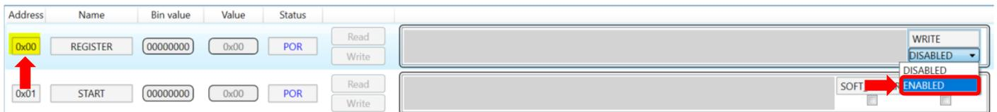
**Figure 19: Select write-protection bit**
